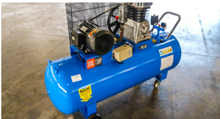
300L Compressor 7.5Hp Motor (x3)
