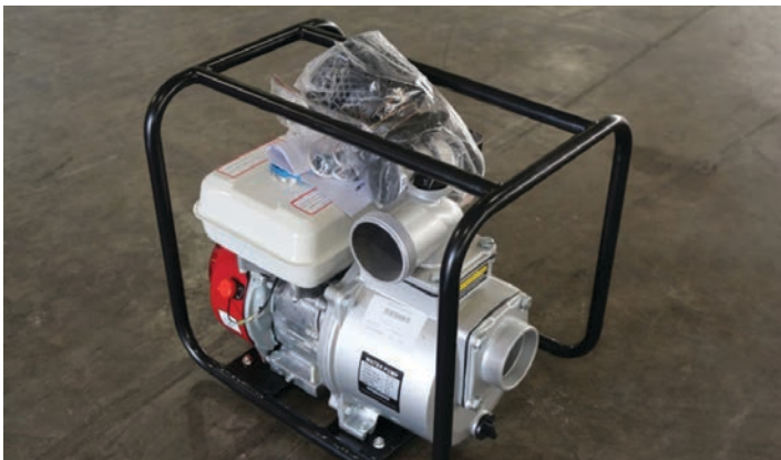
80mm Petrol powered Water Pumps (x2)
