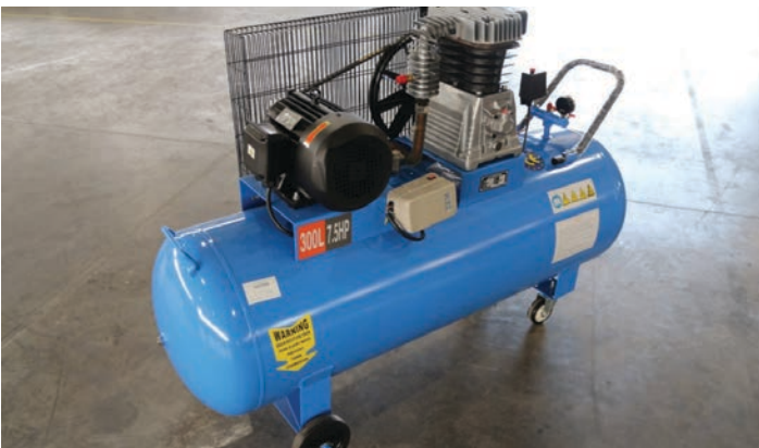
300L Compressors with 7.5Hp Motor (x2)
