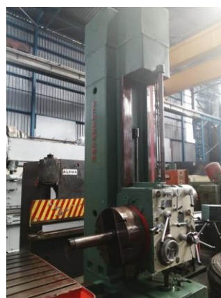
Scharmann 120mm Horizontal Boring Mill with DRO Table 1400mm x 1200mm Vertical Travel 1570mm Cross Travel 1200mm Long Travel 2200mm
