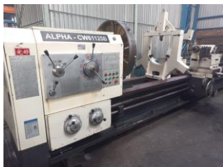
Alpha 8000mm x 1250mm x 130mm Lathe
