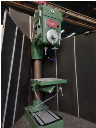
Efamatic 50mm Pedestal Drill - Gear Driven
