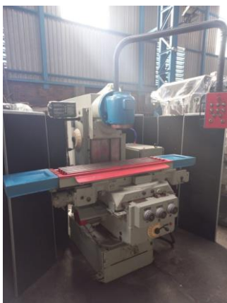
WMW 1250mm x 330mm Milling Machine with DRO
