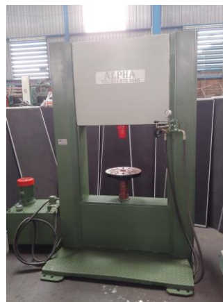
Alpha 50Ton Hydraulic H-Frame Press
