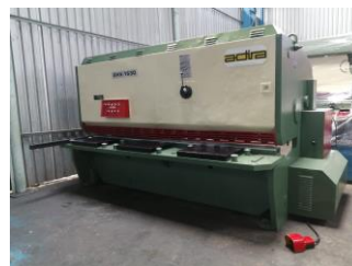
Adira 16mm x 3000mm Hydraulic Guillotine with Motorized Backstop
