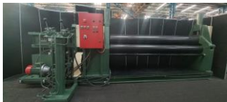
Elga 10mm x 2500mm Semi Hydraulic Pyramid Plate Roller with Section Rolling Attachment
