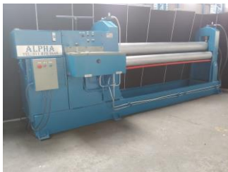
Alpha 6mm x 2450mm Hydraulic Pyramid Plate Roller
