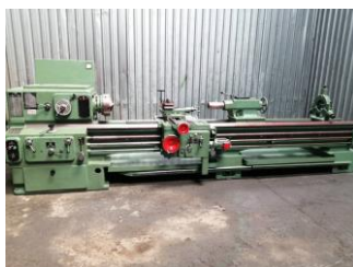
WMW 320mm x 450mm x 75mm Lathe
