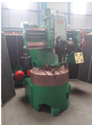
Webster & Bennet Hydraulic Vertical Boring Mill 36", Under Bridge 480mm, Swing 1050mm
