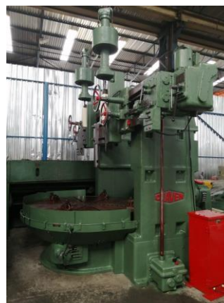
Craven 95" Mechanical Vertical Boring Mill Double Column, Under Bridge 1390mm,
