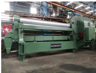
Rushworth 12mm x 3100mm Mechanical Plate Roller
