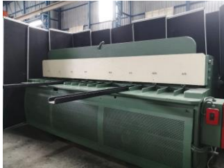
LSG 3mm x 2500mm Hydraulic Guillotine with Manual Backstop
