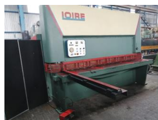
Loire 12mm x 3000mm Hydraulic Guillotine with Motorized Backstop
