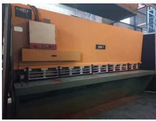
Heli 7mm x 3100mm Hydraulic Guillotine with Manual Backstop
