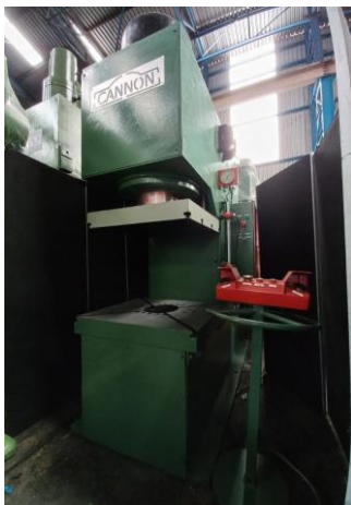
Cannon 320Ton Hydraulic Cushion C-Frame Press 800mm x 660mm
