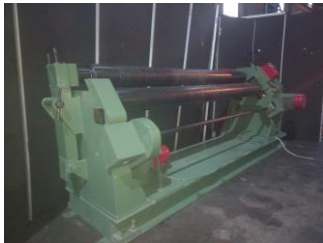
RAB 4mm x 2000mm Mechanical Plate Roller
