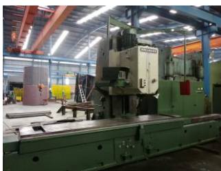
Kollman 4100mm x 700mm Milling Machine with DRO
