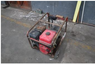
6KVA Generator Faulty
