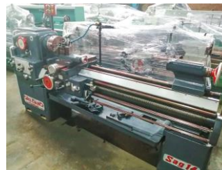
Graziano SAG 14 Lathe 1400mm B/C x 360mm S/O/B x 50mm S/B Location: **Tide Street & Euclid Street, Germiston**
