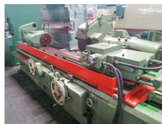
Landis Lunt Internal/External Grinder 2500mm B/C x 360mm Location: **Tide Street & Euclid Street, Germiston**
