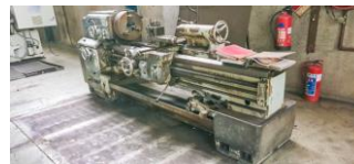
1979 Morando 6100 Lathe with Steady & 3 Jaw Chuck
