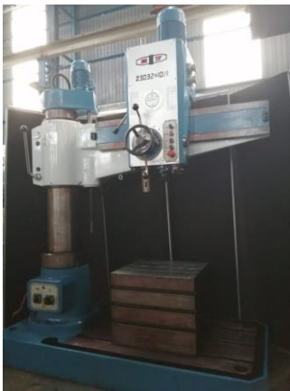
ZJ 32mm Radial Arm Drill, 1000mm Arm Length Location: **Tide Street & Euclid Street, Germiston**
