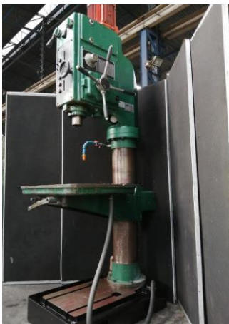
Mitco 50mm Gear Driven Pedestal Drill Location: **Tide Street & Euclid Street, Germiston**
