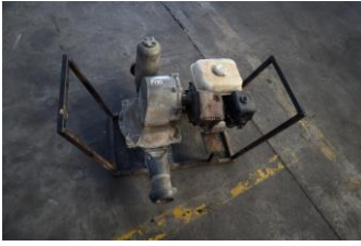
3" Sludge Pump Pump faulty
