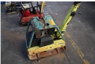
Ammann Forward & Reverse Plate Compactor Engine Seized
