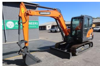
2021 Doosan DX55-9CN Mini Excavator with Front Scraper and Air Conditioned Cab 36.2KW Yanmar Engine VIN: DXCCEADKCM0020858
