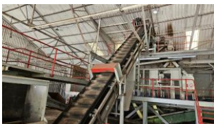
18m Pocket Conveyor with Metal Detector, Pneumatic Flap, Drive Motor, Feed Conveyor and Variable Speed Gearbox
