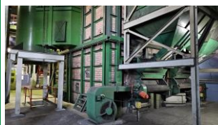
DB Thermal Rotary Dryer with Dutch Coal Furnace, Dual John Thompson Chain Stoker, 2 x FD Fan, Assorted Drum Drives, Control Panel and Assorted Ducting
