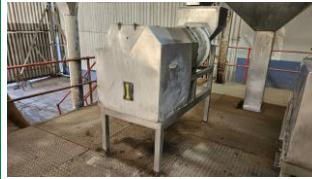
1991 Herbort Dicer Cutting Machine with Aluminum Casing
