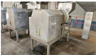
1991 Herbort Dicer Cutting Machine with Aluminum Casing
