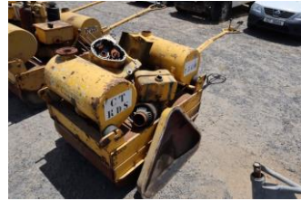
Double Drum Walk Behind Roller Stripped
