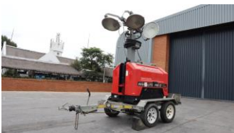
DG80ZXGP Allmand Night-Lite Pro II Double Axle Light Tower Trailer with Caterpillar Engine Hours: 14075 VIN: AA9B116MBEDBE2280 Color: Red
