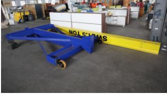
Mobile Gantry Crane and 2Ton Hoist
