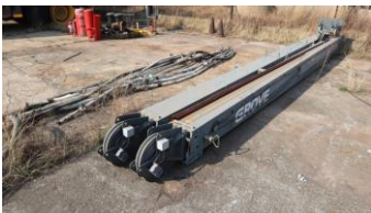
2 x Grove Crane Boom Extensions
