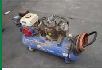
Mac Afric 70L Compressor Faulty
