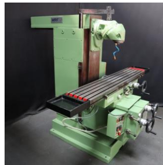
MRF 1,600mm x 320mm Milling Machine
