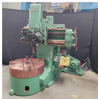
48" Webster & Bennett Vertical Boring Mill with D.R.O. 630mm Under Bridge 1,360mm Swing
