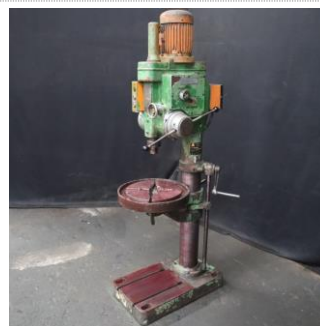
50mm Shang Nong Gear Driven Pedestal Drill
