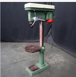
25mm Einhell Belt Driven Pedestal Drill
