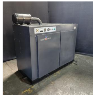
37kW Mutsui Screw Compressor
