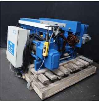
24Ton Munck Motorized Underslung Hoist
