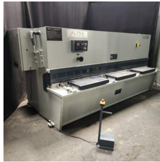
12mm x 3200mm Alpha Hydraulic Guillotine with Motorized Backstop
