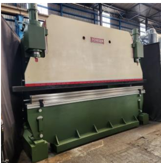
250Ton x 4,350mm Pearson Hydraulic Press Brake
