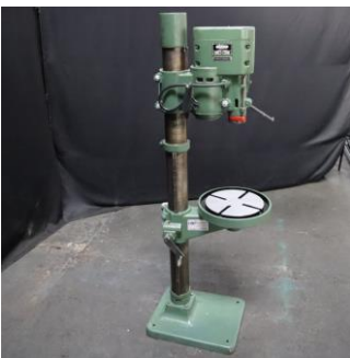
25mm Arboga Gear Driven Pedestal Drill
