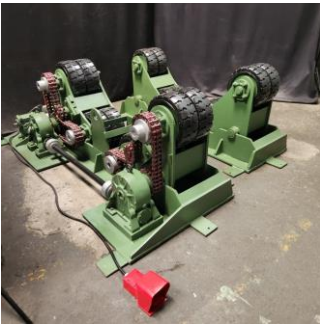
Alpha Motorized Welding Rotator Set
