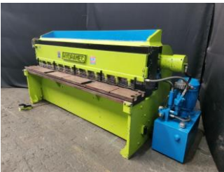
6mm x 2500mm Hydramec Hydraulic Guillotine with Manual Backstop
