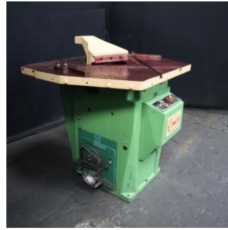
Comaca 220mm x 220mm x 4mm Mechanical Corner Notcher
