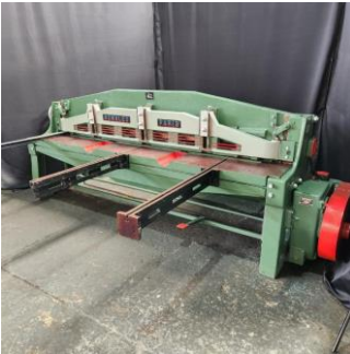
4mm x 2500mm Bombed Mechanical Guillotine with Manual Backstop
