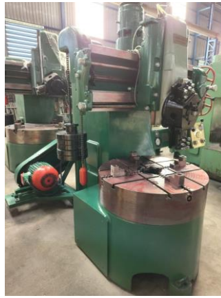
36" Webster & Bennett Hydraulic Vertical Boring Mill 480mm Under Bridge 1,050mm Swing
