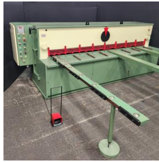
6mm x 3100mm LVD Hydraulic Guillotine with Motorized Backstop
