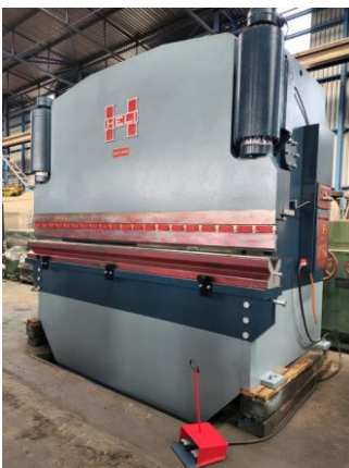
500Ton x 4,000mm Heli Hydraulic Press Brake
