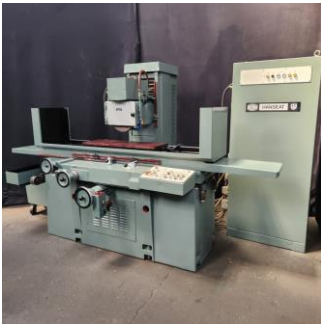
Blohm Surface Grinder with Magnet Size: 900mm x 300mm
