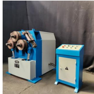
8mm x 100mm x 100mm ACL Hydraulic Section Roller
