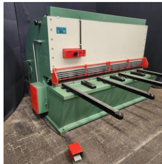
13mm x 2500mm Elga Hydrashear Hydraulic Guillotine with Motorized Backstop
