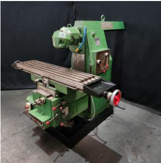
CME FU-1E 1,300mm x 300mm Universal Milling Machine
