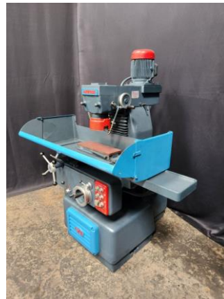
Abwood Surface Grinder with Magnet: 450mm x 150mm
