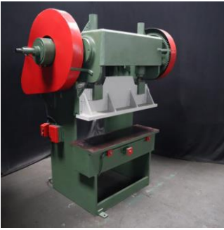
30Ton LSG Eccentric Press with Air Clutch
