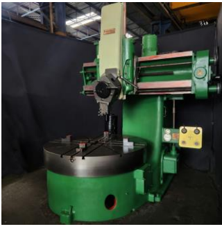
60" Webster & Bennett Vertical Boring Mill 780mm Under Bridge 2,000mm Swing
