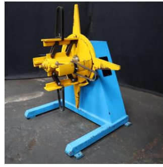
3Ton 200mm wide Coil De Coiler
