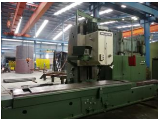
Kollman 4,100mm x 700mm Milling Machine with D.R.O
