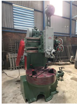
43" Webster & Bennett Vertical Boring Mill 620mm Under Bridge 1,300mm Swing
