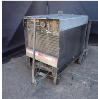
450Amp Transarc Deltaweld 451 Arc Welder
