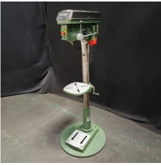
20mm Rexon Belt Driven Pedestal Drill
