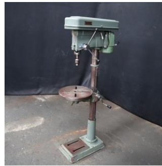
32mm Rexon Belt Driven Pedestal Drill
