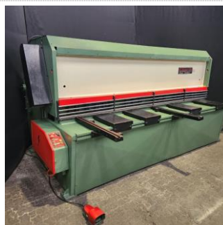
13mm x 3000mm Edwards Hydraulic Guillotine with Motorized Backstop
