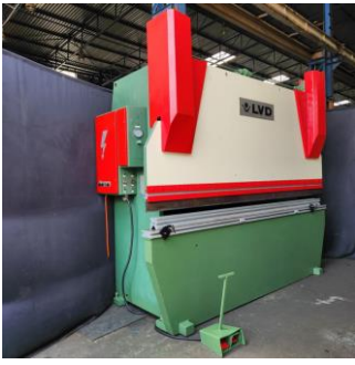
165Ton x 4,000mm LVD Hydraulic Press Brake
