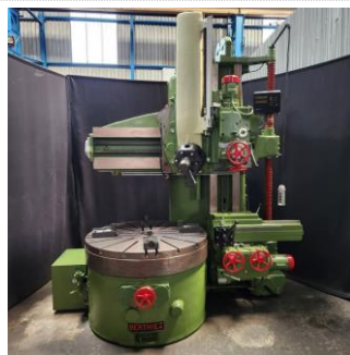
55" Berthiez Vertical Boring Mill with D.R.O. 1,200mm Under Bridge 1,600mm Swing
