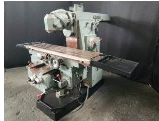
Correa FU3E 1,400mm x 340mm Universal Milling Machine
