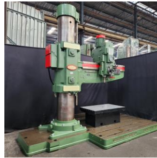
100mm x 2,000mm Asquith OD4 Radial Arm Drill 3,000mm x 3,000mm Table
