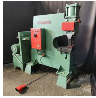
Peddinghaus 225H/65 Hydraulic Punch 22mm x 22mm, OR 27mm x 19mm
