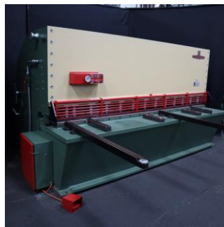
13mm x 3000mm Elga Hydrashear Hydraulic Guillotine with Motorized Backstop
