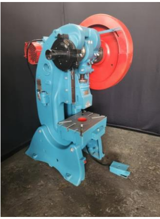
40Ton HME Eccentric Press with Adjustable Stroke and Air Clutch
