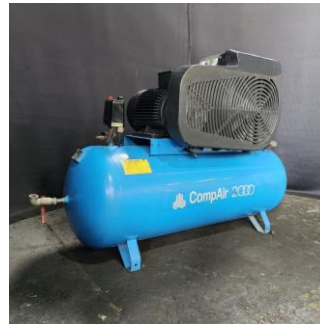
7.5kW Compair 2000 Compressor
