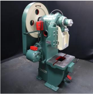
30Ton Caxton Eccentric Press with Adjustable Stroke
