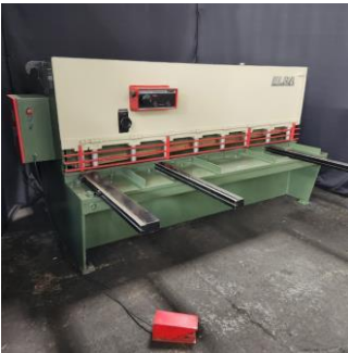
6mm x 2500mm Elga Hydrashear Hydraulic Guillotine with Motorized Backstop
