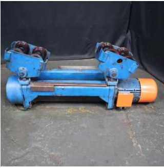
10Ton Misia Underslung Hoist
