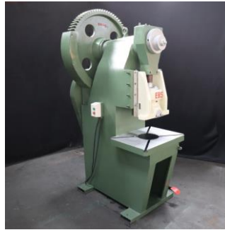
65Ton EBS Eccentric Press with Adjustable Stroke
