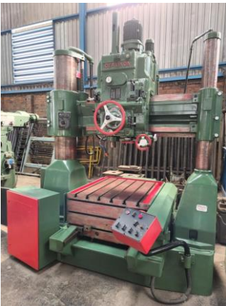
55mm x 1,350mm Oerlikon Radial Arm Drill 1,000mm x 1,000mm Table
