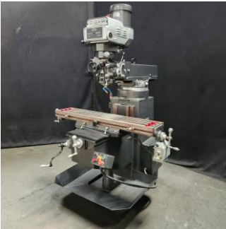
Bemato 1,270mm x 255mm Turret Milling Machine
