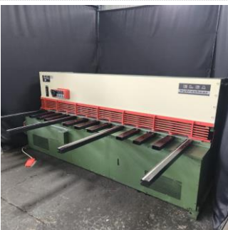
6mm x 3000mm Elga Hydraulic Guillotine with Motorized Backstop
