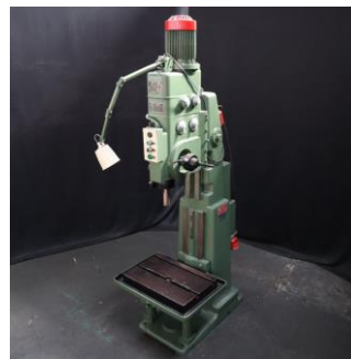
35mm Elliot Elevating Head Gear Driven Pedestal Drill
