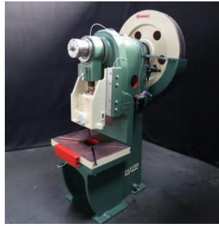
60Ton Caxton Eccentric Press with Adjustable Stroke
