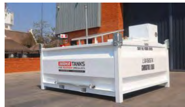
WAHA 4,500L Self Bunded Solar Fuel Tank With Batteries and DC pump Self bunded with internal tank and external bund. Corner container lock castings. Internal ladder for access Three 600mm manholes Air breather vents for free venting Containment compartment (internal bund) with emergency vent. Calibrated contents dip stick Top roof section designed to release water Paint coating to c5-1 harsh environment standard, three coats Hempel paint to 240 micron thickness. with 150W Solar Panel
