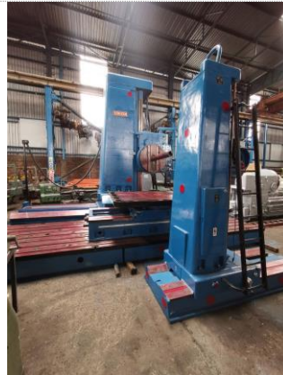
2008 Union BFP160 160mm Spindle Floor Borer with Rotary table and D.R.O 160mm spindle 2300mm x 2000mm table size 2000mm vertical travel 1500mm cross travel 3200mm long travel
