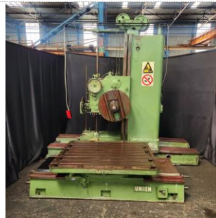
Union BFP125 125mm Spindle Horizontal Boring Mill with Rotary table 1900mm x 1600mm table size 1550mm vertical travel 2300mm long travel
