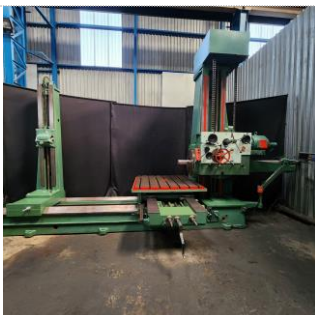
Collet 115mm Spindle Horizontal Boring Mill with D.R.O 1600mm x 1400mm table size 1900mm vertical travel 1650mm cross travel 2600mm long travel
