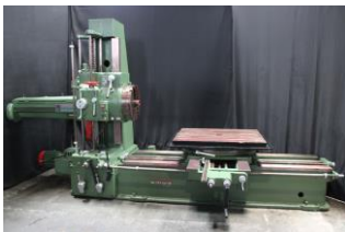
Union BF80 80mm Spindle Horizontal Boring Mill 1120mm x 900mm table size 900mm vertical travel 1000mm cross travel 1700mm long travel
