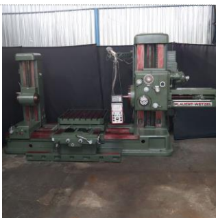
Pluert Wetzel 100mm Spindle Horizontal Boring Mill with D.R.O 1430mm x 1280mm table size 1100mm vertical travel 1100mm cross travel 2000mm long travel
