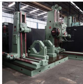
Skoda HVP160D 160mm Spindle Floor Borer 160mm spindle 4485mm x 1750mm table size 1900mm vertical travel 5000mm long travel
