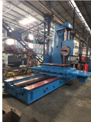
Union BFT125/5 Horizontal Boring Mill 1600mm x 1400mm table size 2000mm vertical travel 1600mm cross travel 2000mm long travel
