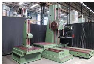
Scharmann 160mm Spindle Floor Borer 160mm spindle 3400mm x 1525mm table size 2600mm vertical travel 5000mm long travel D.R.O. Rotary table –
