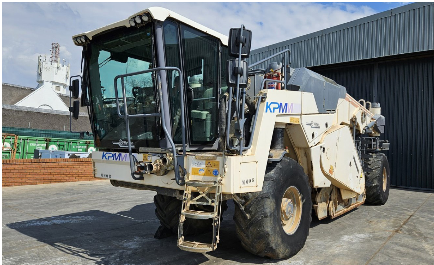
2015 Wirtgen WR2000 Cold Reclaimer/Recycler
