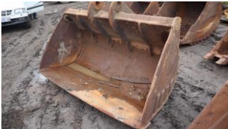
20Ton Excavator Coal Bucket
