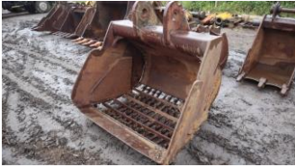
20Ton Excavator Grid Bucket
