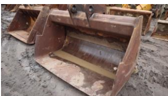
20Ton Excavator Bucket
