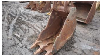
Excavator Trenching Bucket
